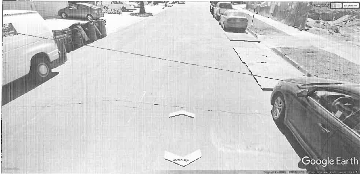
Figure 7 Fault runs across Malcolm into site. Roadway cracks from surface faulting run into site.
