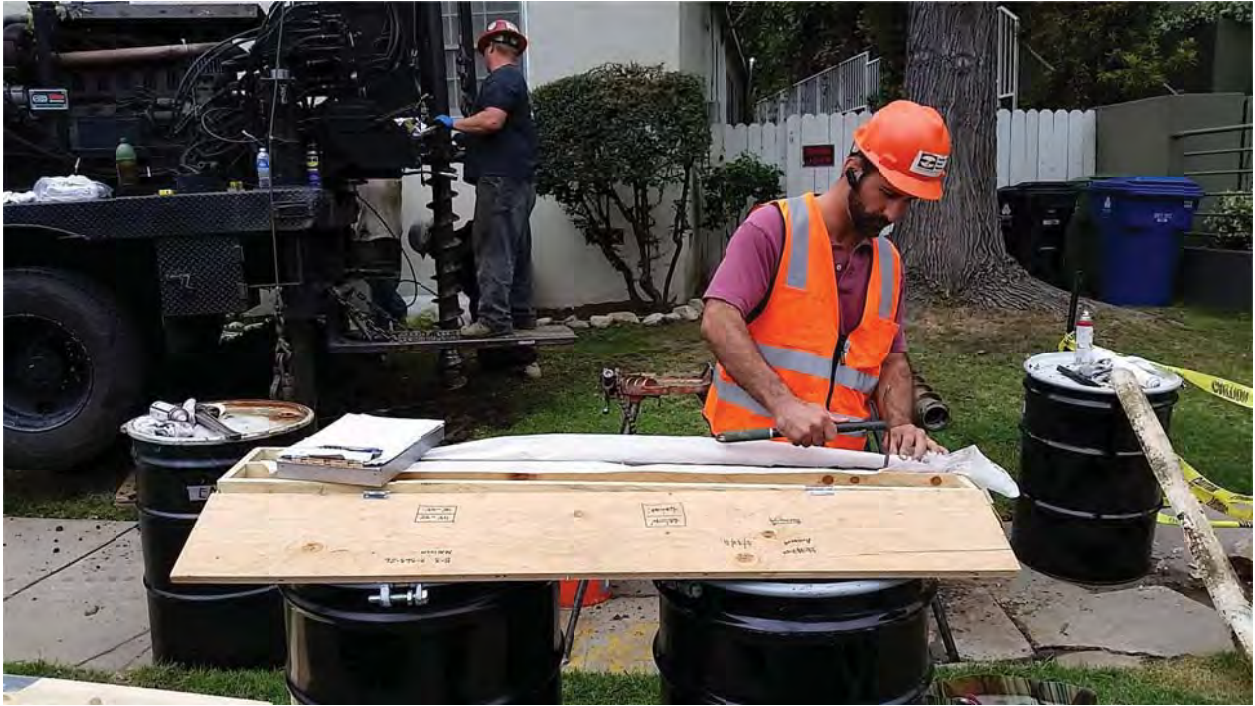
Photo 2: Shant Minas, Engineering Geologist, Logging Core Samples from B-3. Note Large Tree and surrounding earth mound which complicated drilling in the area north of B-3.
