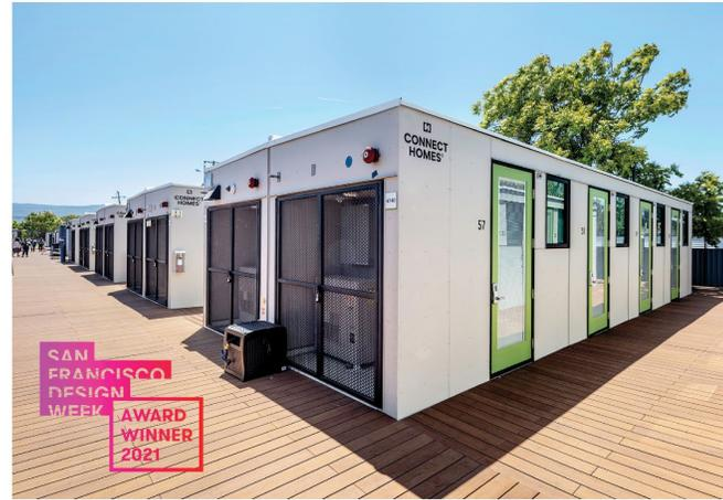
Connect Shelters come in multiple configurations and fire-resitant wall assemblies mean they can be placed back-to-back and/or stacked for increased density.
